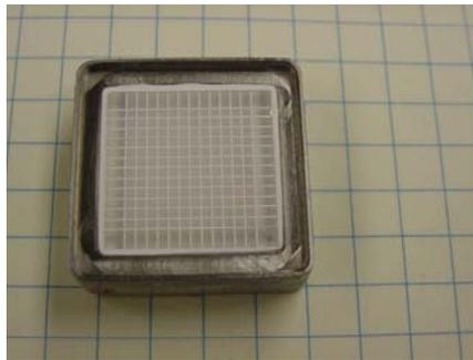
Figure VII: 1" square NaI(Tl) Crystal. Note the wider crystal around the edge and glass that seals the crystal
